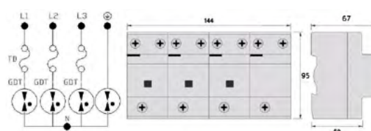
AA4-H100 electrical diagram and dimensions
