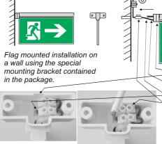
5. Place the mounting accessories in the wall and screw the mounting screws
