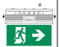
NOTE!! After finishing the installation you must power the luminaire for at least 24 hours for battery charging to perform the nominal autonomy.
