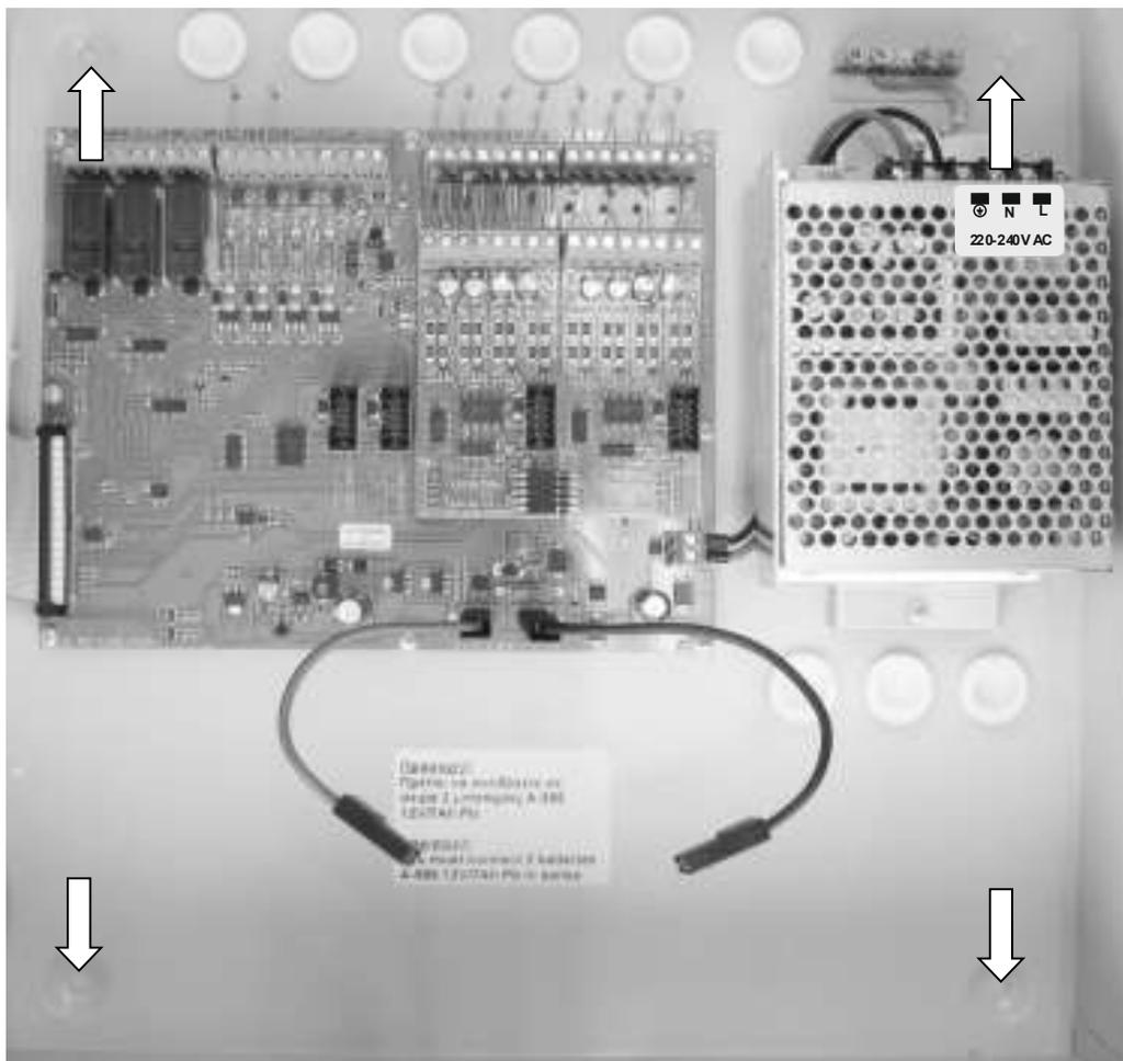
Figure 4-20. Mounting hole locations.
