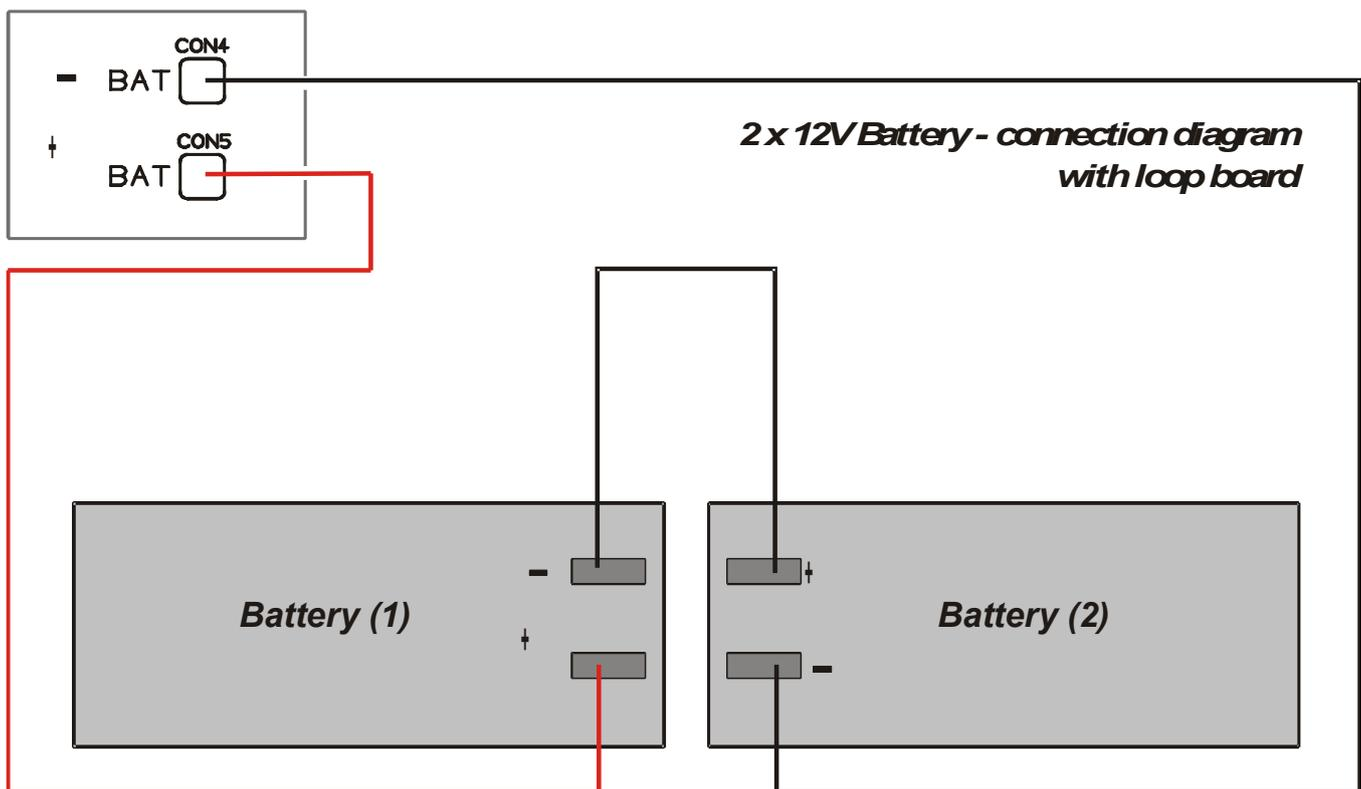
Figure 4-23. Connecting the batteries in series.
