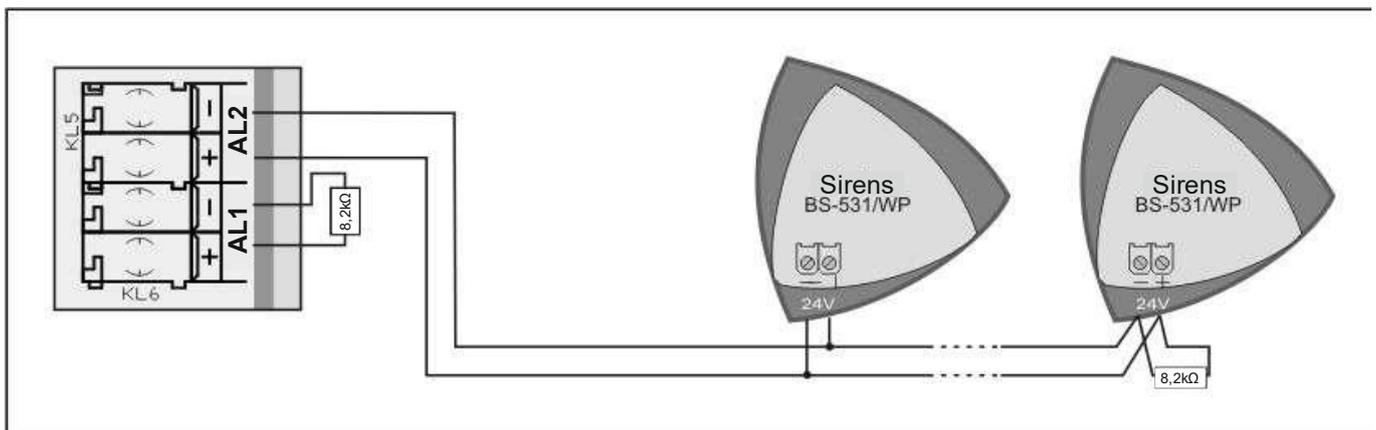
Figure 4-27. Connecting the sirens to the panel
