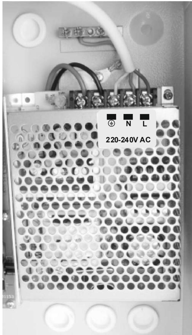
Figure 4-22. Connecting the 230VAC
