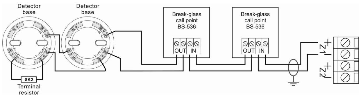
Figure 4-25. Connecting 2 detector bases and 2 BS-536 call points to zone 1. On each base you can install BS-655, BS-660 or BS-657 detectors.
