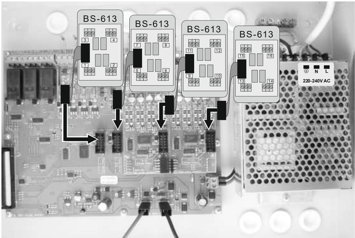
Figure 4-28. Relay per BS-613 installation
